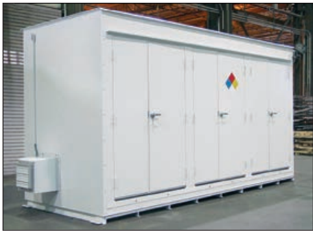
Chemical Storage Locker with 2-hour fire rated design features three door sets to ease material handling. Order No. N05-4040
