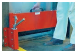
At the first sign of an incident the barrier is lowered into position.
