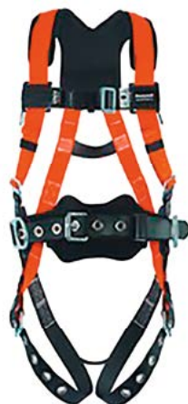
Harnesses with back&side D-ring&tongue-buckle legs, soulder/waist padding&remov.tool belt, Order no. M74-2982-U0
