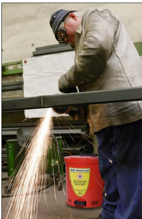
The self-closing lid prevents the content from igniting, e.g. by flying sparks
