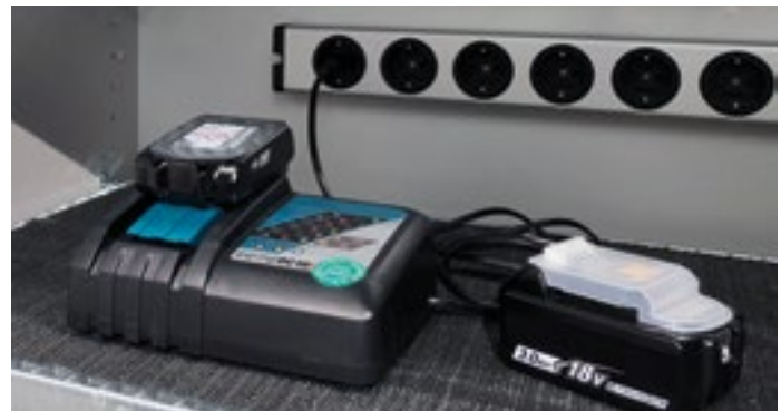
Charging station in safety cabinet
